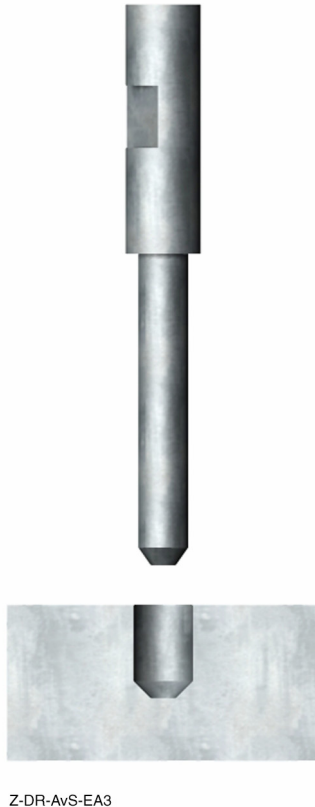
Figure 7-1: Stud and plate geometry used for parameter influence experiments.
