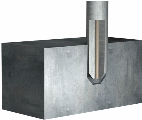
Figure 7-8: Stud design with nickel tracer rod.
