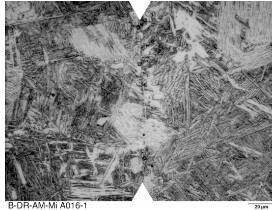
Figure 7-53: Microstructure in region J, bonding line indicated by arrows (original magnification: 500x).
