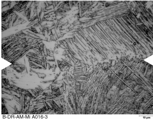
Figure 7-45: Microstructure in region B, bonding line indicated with arrows (original magnification: 1000x).
