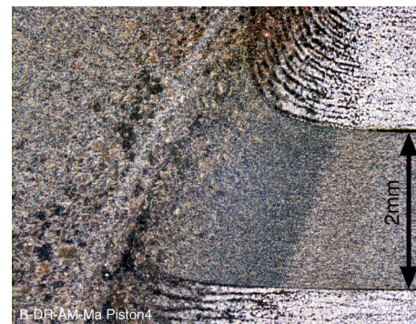
Figure 7-70: Plastic deformation of piston 4 (2 mm diameter) at the bonding line interface in a tapered weld. Owing to the welding forces and temperatures associated the tip of the piston is plasticised and deformed.
