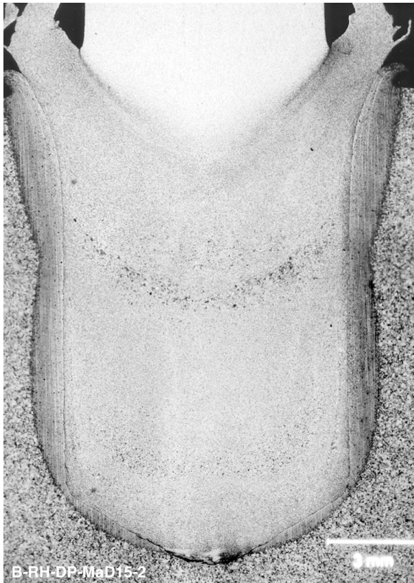
Figure 3-2: State of the art FHPP weld. (DIN S235 Mild steel stud in a S690QL CrMo steel plate).
