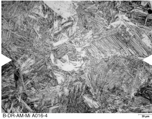
Figure 7-44: Microstructure in region A, bonding line indicated with arrows (original magnification: 500x).
